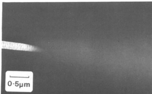
Figure 4 Blunting by shear at the tip of a long craze in PS:PPO 1.
